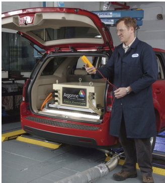
A researcher at Argonne National Laboratory checks a plug-in hybrid electric vehicle battery. As the technologies develop and become more available, national energy policies can create incentives to purchase electric vehicles.
